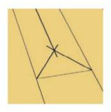
Saw through the damaged board along its central line. Saw a "V" at each short end.
