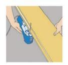
Cut off the tongue on the long and short sides. Lightly sand (0.5 mm) the tongue to allow room for the adhesive.
