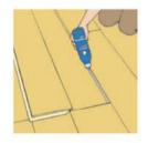
Apply adhesive to the underlips of the surrounding boards and the replacement board.
